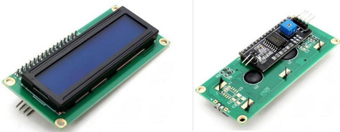
This can display is a 16 character x 2 lines version but bigger displays can easily be incorporated as required.
