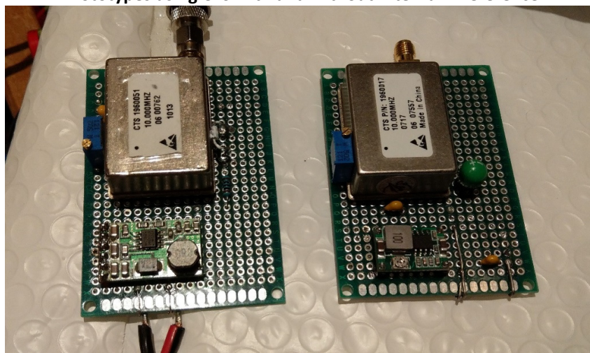
Prototypes using CTS with and without Internal V reference
