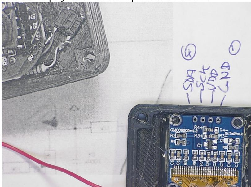
Also, after testing to make sure the connections are correct, apply some hot melt glue to anchor the wires.
