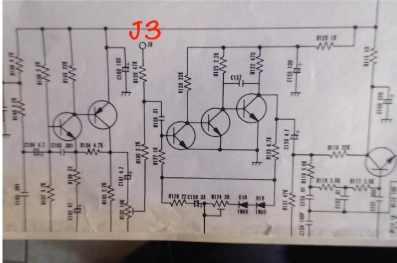
The CTCSS injection is this point on the circuit...
