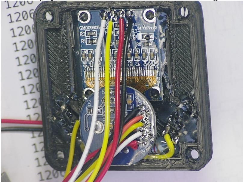
A hint, write down the display connections as seen from the back as when the display is mounted, the labels cannot be seen, and not all displays are the same. Guess how I know?? Also, not all OLED displays have the same pinout!! Be careful.
