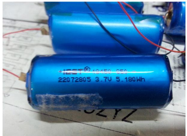
Do not short the battery wires unless you want some fire! I did and it is pretty spectacular. Cut the red from the battery, then the black. If you want, the pressure switch and heater can be salvaged too, along with any other parts you want. But I am just interested in the battery.
