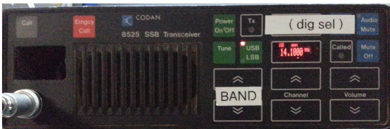
The “Clarifier” buttons are used for the band selection now., while “Channel” is the tuning. “Scan” and “S/Call Mute” are the digit select < and > respectively.
