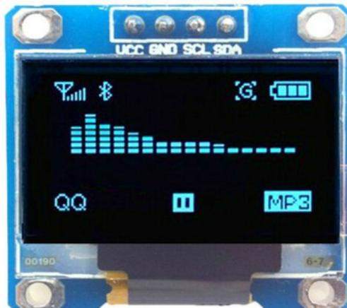
Both use I2C 2 wire communication driven from the Arduino.
