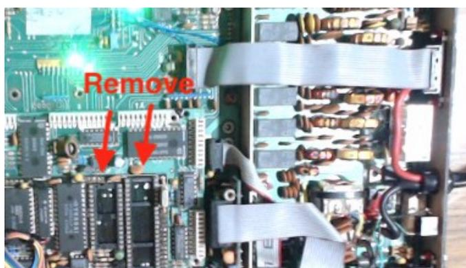
Also, remove the front panel so the original display board can be discarded (in the safe place with the CPU and EPROM).
