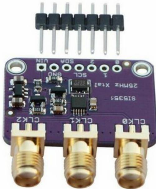
The outputs can be taken from pins 0, 1 and 2, but I use coax cables screwed to the connectors supplied, and they solder to the CLK0 – CLK2 positions.
