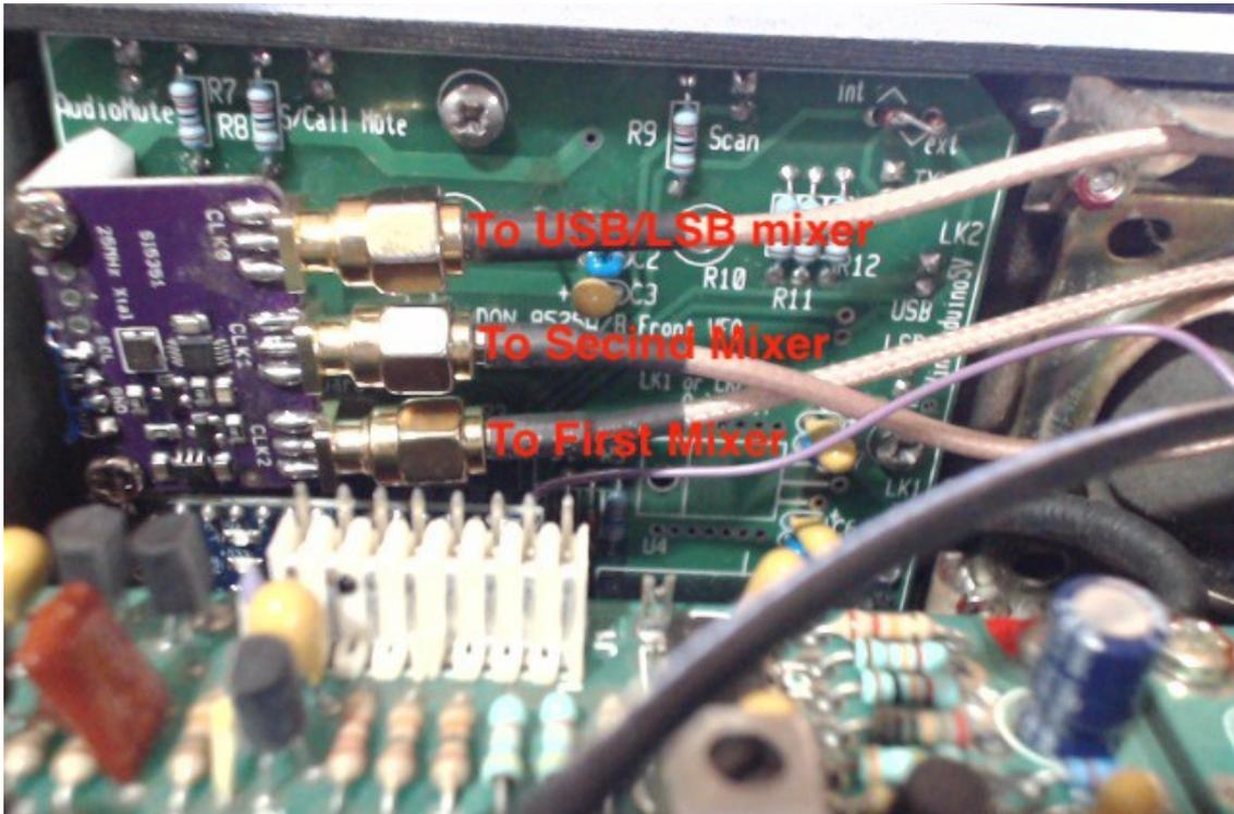
There is wire running from the VFO to the Codan controller board for the Tune signal. It is just pushed into the connector as below.
