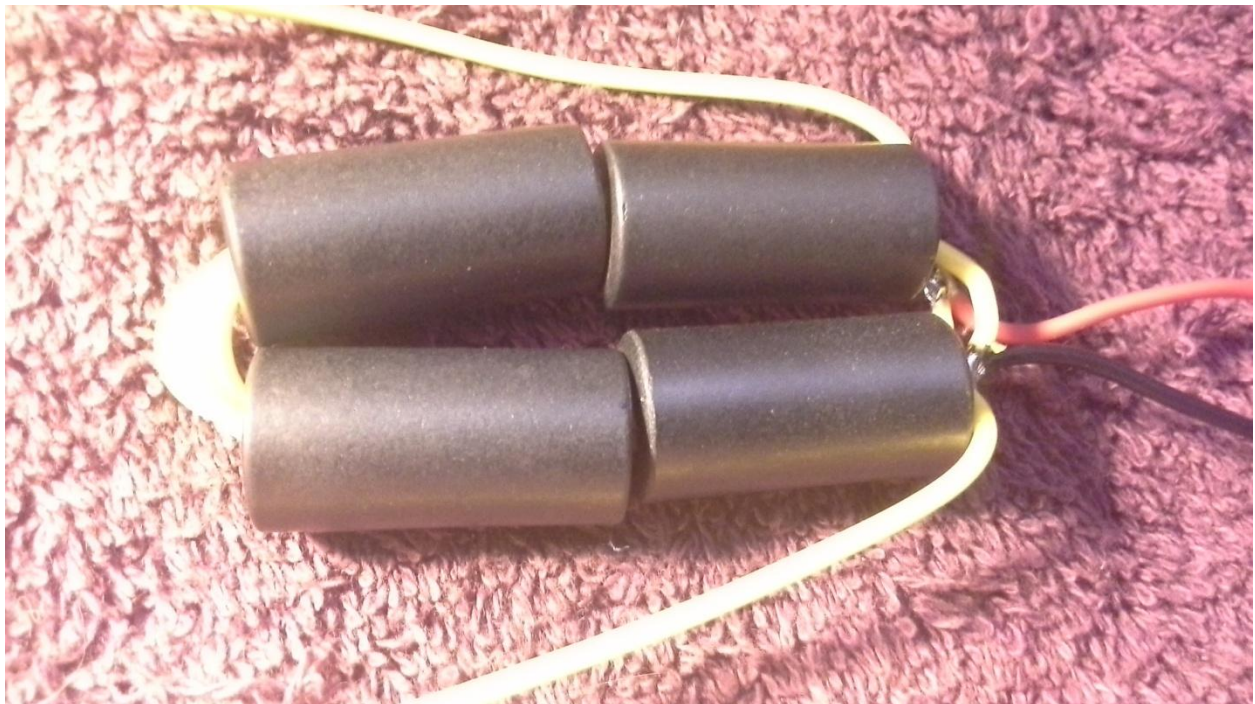
Pull one pass back out of the cores of the original design to make it 3 passes for a 9:1 Balun.
