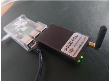
Allstar is a means of conversing with digital voice over the internet from an FM amateur handheld radio to another Allstar node anywhere in the world. It provides direct amateur to amateur call and connection to nets including some connected to FM repeaters.
