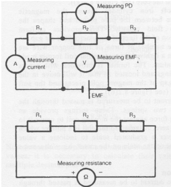
**Figure 8.1** Voltage, current and resistance measurement
