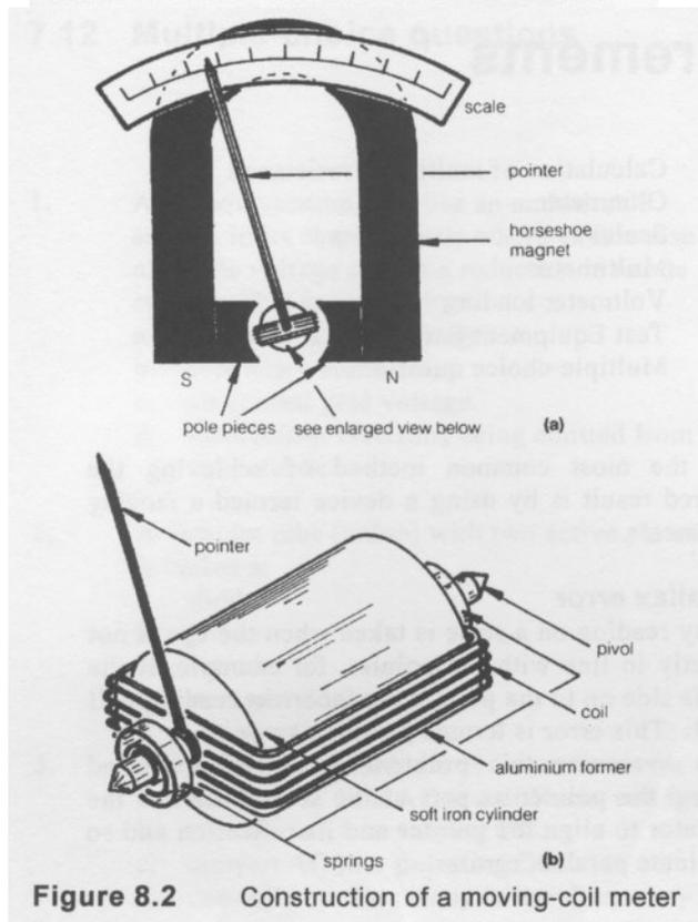
**Figure 8.2** Construction of a moving-coil meter
