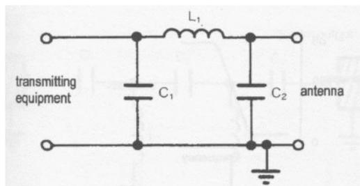
Low Pass Filter circuit. Notice the similarity to the above circuit.
