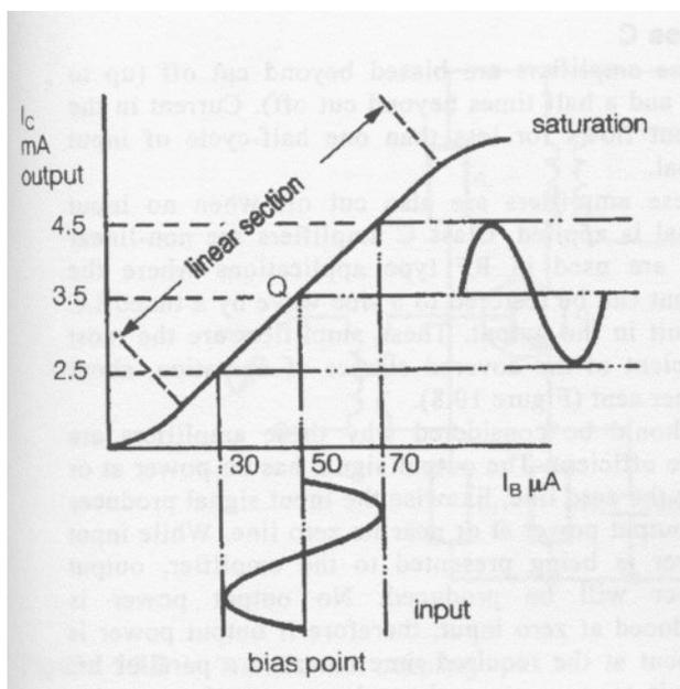
Q is the most linear point on the load line of the above graph.
