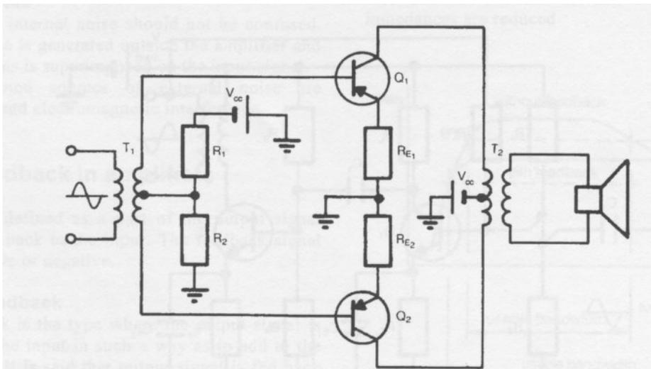
The above is a push pull amplifier operating in class B configuration.
