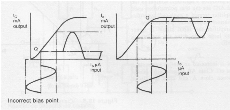
Incorrect bias points for proper linear Amplification.
