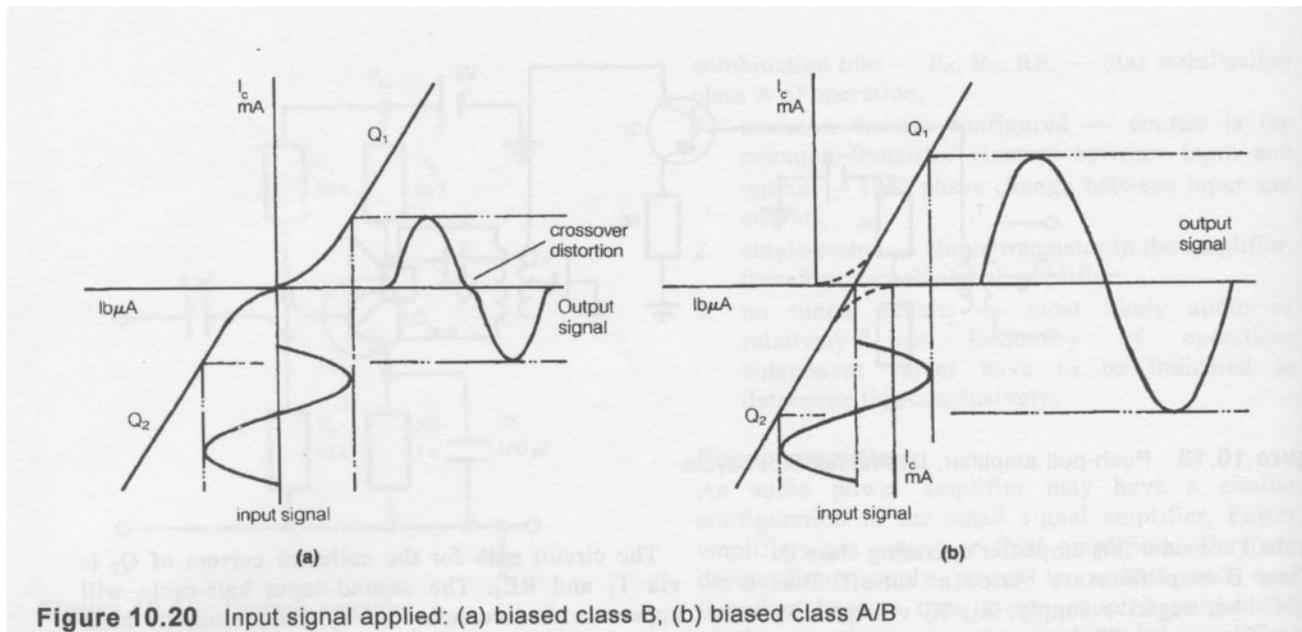
**Figure 10.20** Input signal applied: (a) biased class B, (b) biased class A/B
