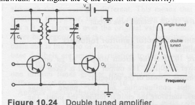
**Figure 10.24** Double tuned amplifier
