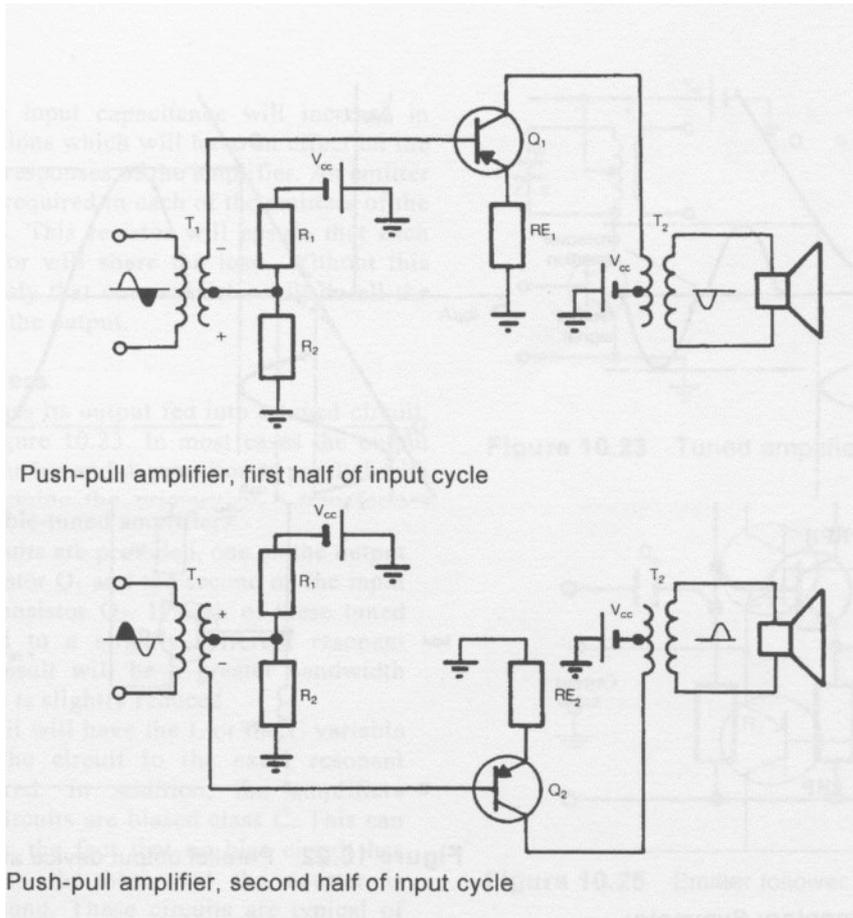
The push pull amp has only 1 transistor operating per half cycle of the waveform input, thus operating each transistor only half the time, ie 50 % duty cycle.
