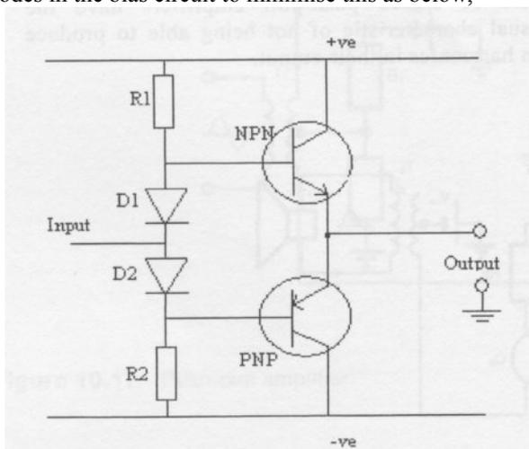
The diodes offset the transistor junction voltage drop by 0.6 volts to produce a more linear and less distorted output. See graphs below,
