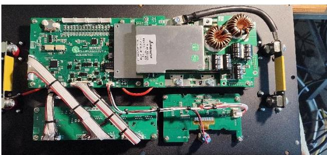
The selection of a BMS has more to do with the maximum magnitude of currents that battery is to handle. For example you wish to have an energy store of 1 KWh but will only draw 10 Amps and charge at 50 Amps, so the BMS has to cope with 50 Amps maximum, but give yourself a bit of head room selecting a 100 Amp BMS, you can use a larger capacity BMS but not one that is smaller.
