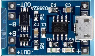
This version, with the B-, B+,OUT- and OUT+ has charge and discharge protection. There are some that are only chargers, but I would go with the boards that have both.
