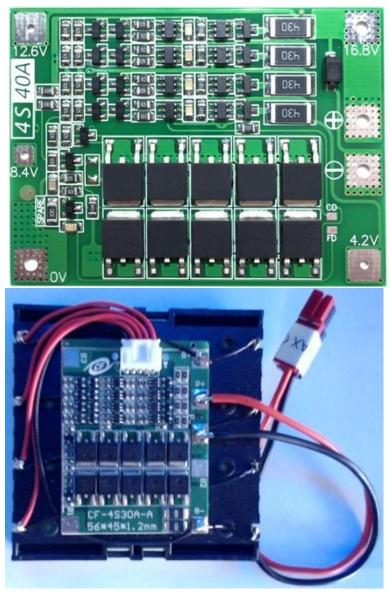
For multi cells in series, a board that also includes cell balancing is needed. This and other versions can be found for under \$15 from Ebay.
