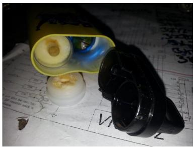
The case is Aluminium with the ends pushed in. Grabbing the mouth piece with pliers, and applying a bit of brute force, it can be
