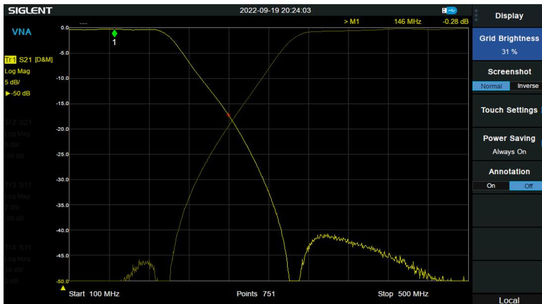
The rejection of the unwanted band in both cases is around 50 dB, the insertion loss is about 0.3 dB Return loss ( VSWR ) was better than 1.1 :1 on all three ports.
