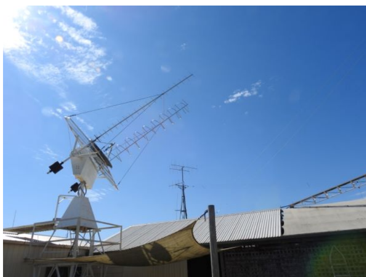
A fully rotatable vertical and horizontal direction and polarisation ISS control station antenna system - VK5ZAI at Kingston South Australia
