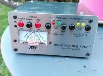
It has a simple algorithm programmed into it to stop and beep when a "dip" in reflected power is recorded.
