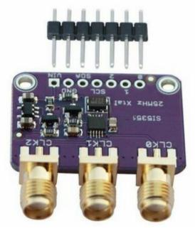
The outputs can be taken from pins 0, 1 and 2, but I use coax cables screwed to the connectors supplied, and they solder to the CLK0 – CLK2 positions.
