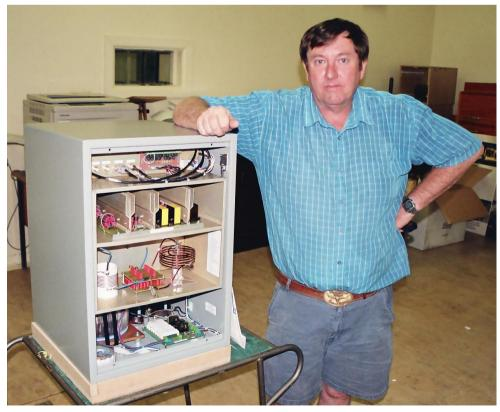
Terry Fahey at Radio Australia in 2007 inspecting a fully solid state 1 KW Blythe **Broadcast Band** transmitter. The Radio Australia staff looked after a number of small broadcast band transmitters as well as the 100 KW transmitters on site.
