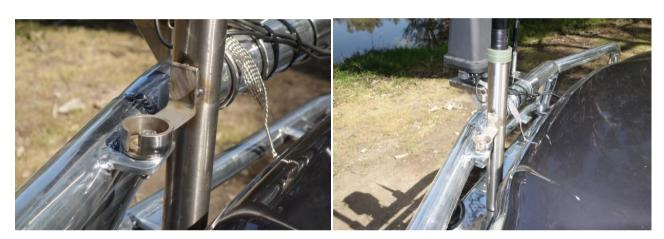
The tube mount can be removed when not required but can also be left on when moving around as it's very sturdy and doesn't move once fitted. Because the squid pole is very light, the wire can be wound around it helically on the ground and it can be lifted into position into the tube where it sits steady as I have made up a round plastic bush stabiliser for the squid pole and the top of the steel tube mount. This steadies the pole to stop it flopping around needlessly.
