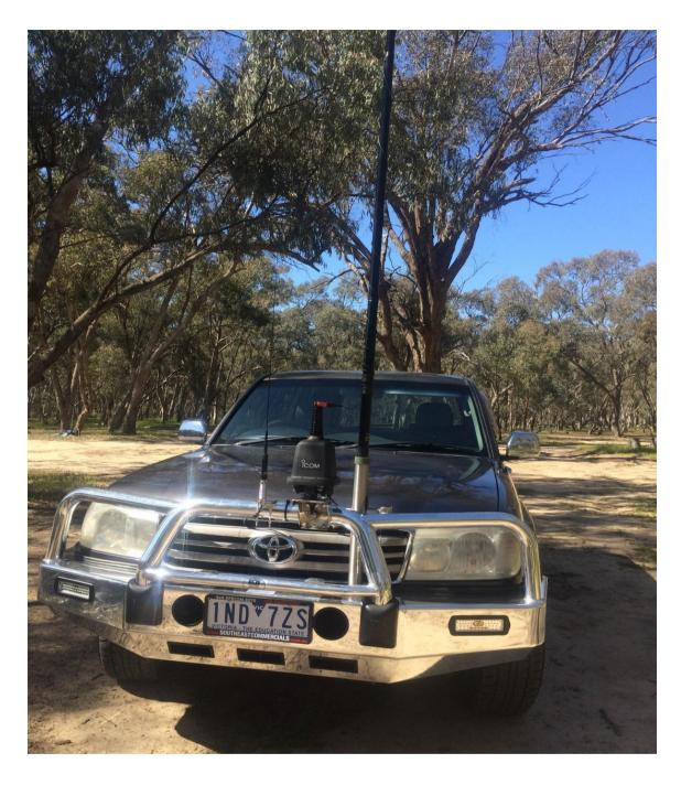
The squid pole and vertical antenna is very good out in the bush where there is little man made noise and makes for a great portable operating experience. Anywhere the vehicle can get to, the portable station can be set up.
