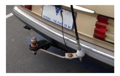
Huntly VK3ZE saw this installation recently in a Shepparton car park. It is a novel way of mounting an antenna on the tow bar of your car using a large ring spanner. How well it works we don't know. Is the installation for 27 MHz CB or HF amateur bands? The earth path is the main concern.
