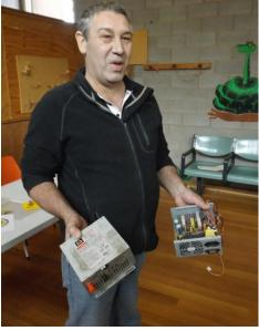
Rodney VK3UG showed his prototype power supply used to power vintage battery powered radios. It has a capability of supplying 20 different voltages of which 14 are available at any one time. It has a number of active and passive voltage and current regulators to achieve the required voltages at different current capabilities.
