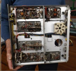
Phil VK3ELV showed us a power supply that he has modified for amateur use. His little project at the show and tell was an old computer power supply converted to a 13.8v supply to run a transceiver.
