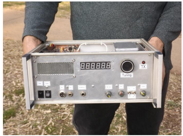
A front panel view of the 40 metre transceiver with a digital frequency readout.
