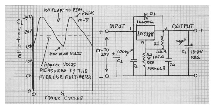
The value of the output filter capacitor C2 is not particularly critical but I would suggest around 100  $\mu$ F per amp of output current.
