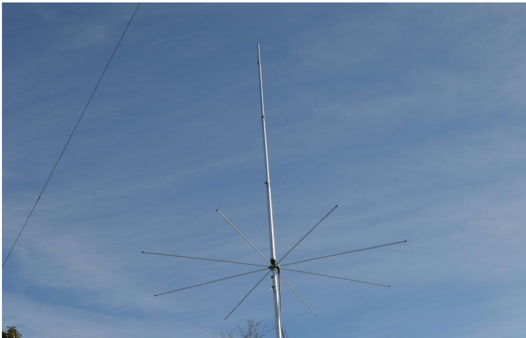
The antenna mounted at the QTH. The elements are quite thick on the radiator to give a wide Bandwidth. The XYL can now hang the washing on the antenna radials!! She's a little disappointed that the radials don't spin around on a windy day...☺
