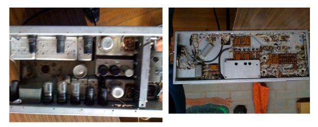
These pictures give some idea of the complexity of the unit. The unit is a 105A/ARR-15 receiver. It was designed for use as an auto tune unit in combination with the autotune ART-13 transmitter. The receiver can be manually tuned if you lock the autotune mechanism and you can also manually tune the transmitter in a similar manner.
