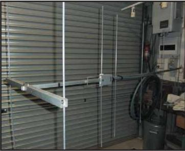
The first two metres of feedline is also protected by being inserted into twelve millimetre water hose. This is the 2 metre yagi.
