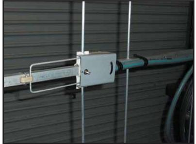
In an attempt to lessen the damage caused by Corellas I have covered the feedpoint with a guard made from thermoset plastic. This is simply a piece of UV proof stormwater pipe tested in the microwave oven for suitability before heating with a heatgun and molding into shape
