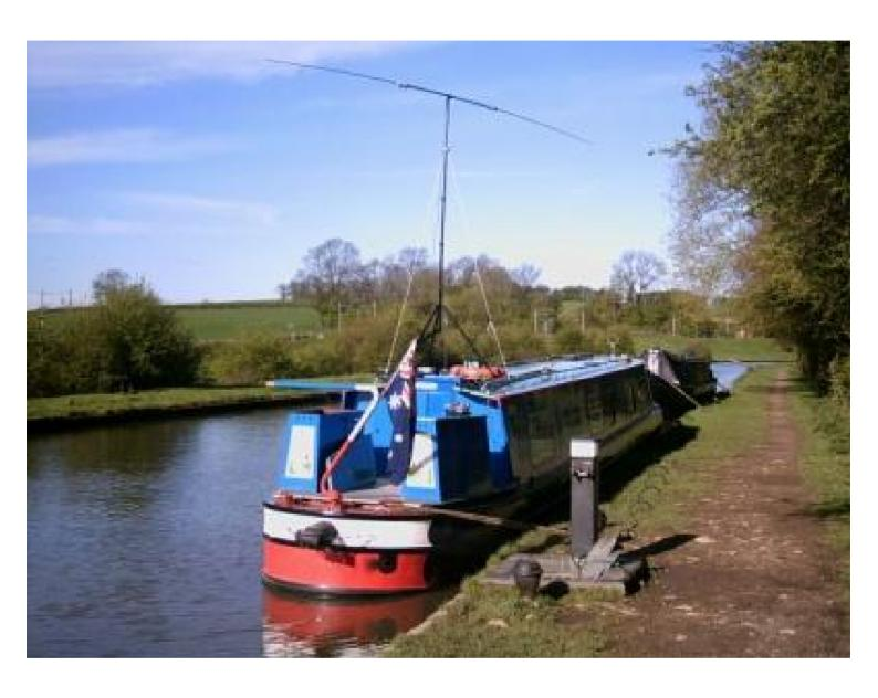
Roger M/VK2RO/MM Grand Union Canal Warwickshire England, Equipment Buddipole Dipole on 20mts, Rig Icom IC-706 MK11G, Long Boat 70ft Steel Hull, 4 cylinder lister diesel engine, 7mph top speed, 25 Tons loaded full 4 star rating.
