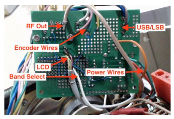
The rotary encoder is mounted in the "CLARIFIER" hole. An unused hole, "MUTE", was enlarged a bit to fit the USB/LSB switch.
