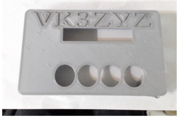
This front will (hopefully) be held in position with magnets. The 4 large holes let the sound out.
