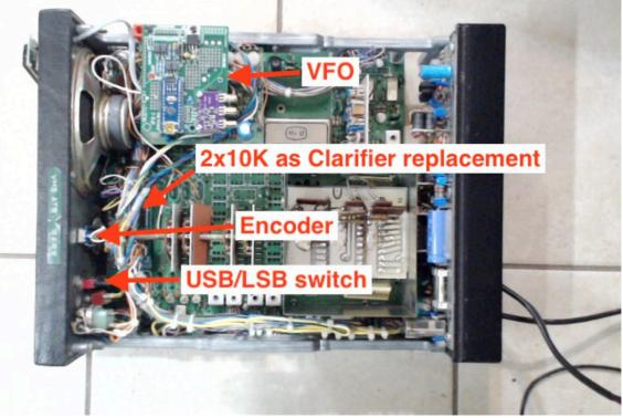
Wires are just soldered on, and the coax connectors are not used. These could be left off the Si5351 board.
