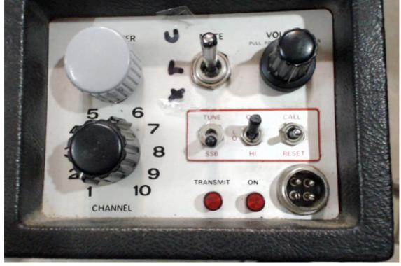
I had removed the clarifier pot, so replaced that with a couple of 10K resistors with heat shrink around them for protection.
