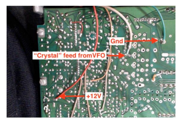
T Connections to the main transceiver board are as follows...
